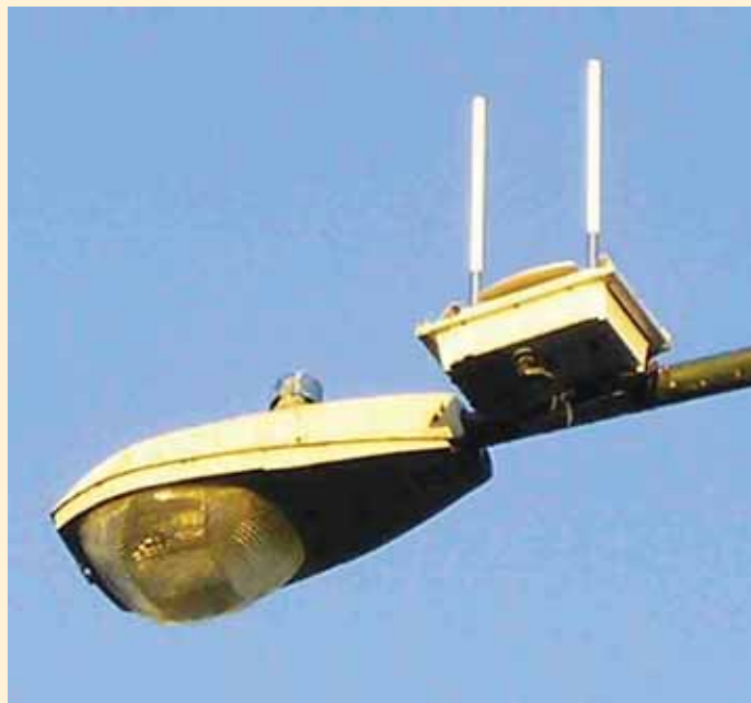
A Google access point, located on a Mountain View lamp post.
