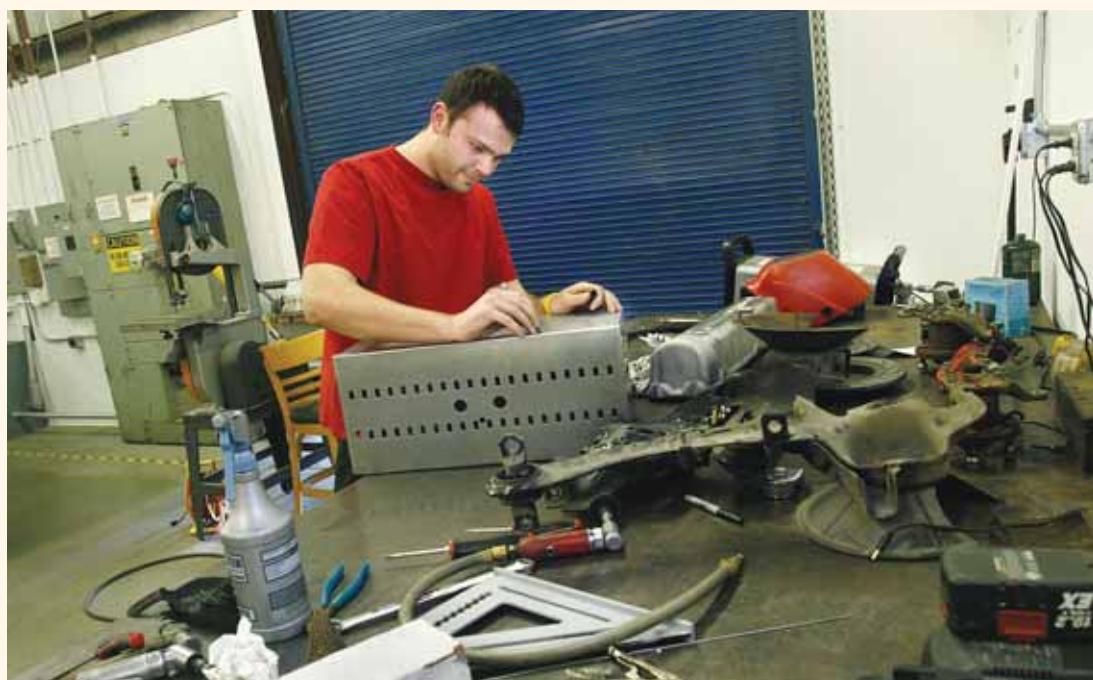
Morgan Gillis constructs a battery box for a Kleenspeed Technologies race car. Below: A former Spec Racer Ford fitted with an electric drivetrain.
