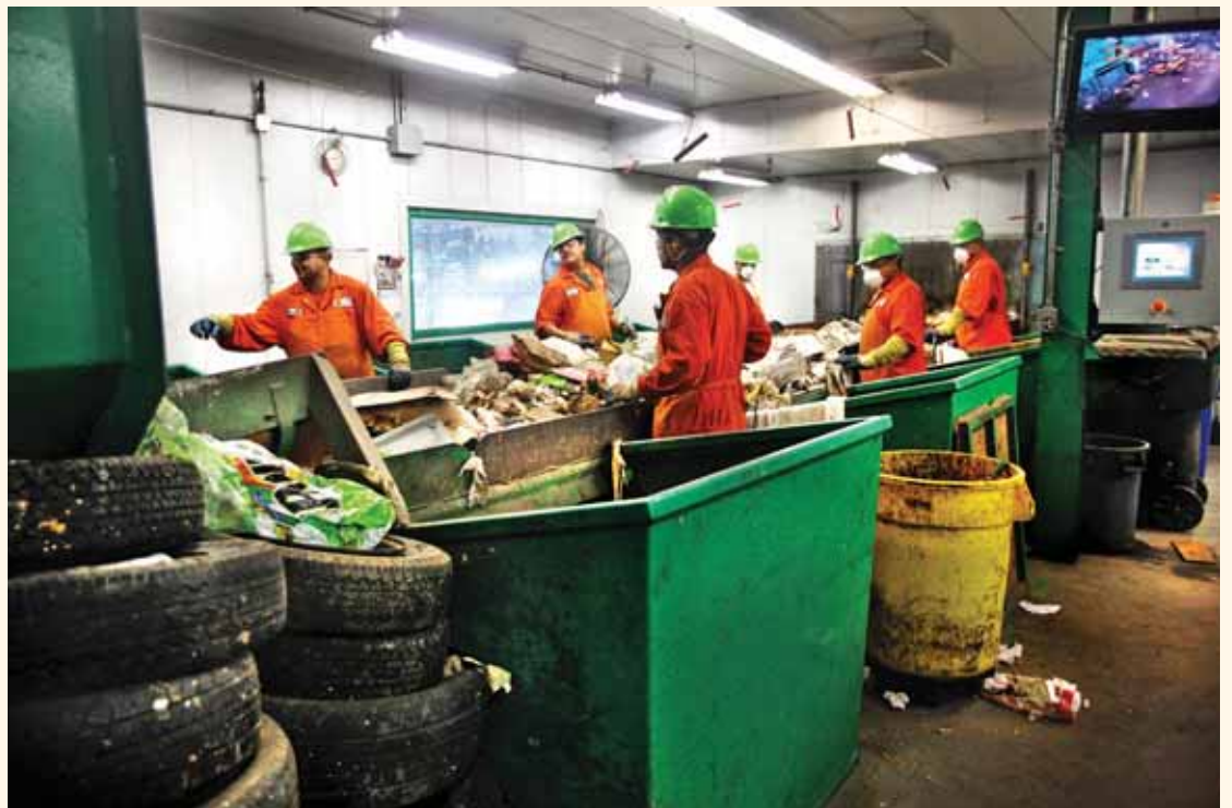
Workers at Sunnyvale's SMaRT Station manually remove cardboard, wood and large objects from a conveyor belt leading to mechanized garbage sorting equipment.
