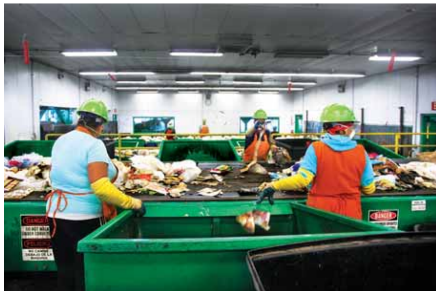
A group of workers manually sort garbage at Sunnyvale's SMaRT Station, removing paper, cardboard and other recyclable materials.
