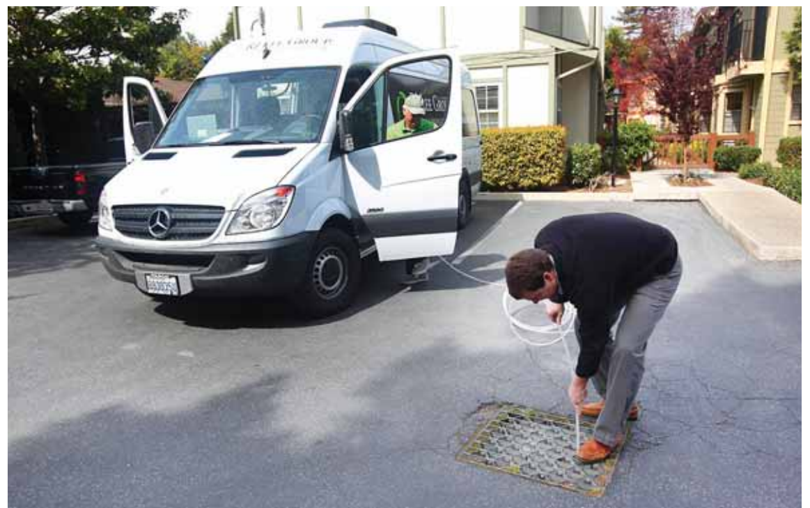
Todd Rogers collects an air sample using a Teflon tube connected to a van owned by the R.J. Lee Group, which is demonstrating an instrument that measures toxic vapor levels.
