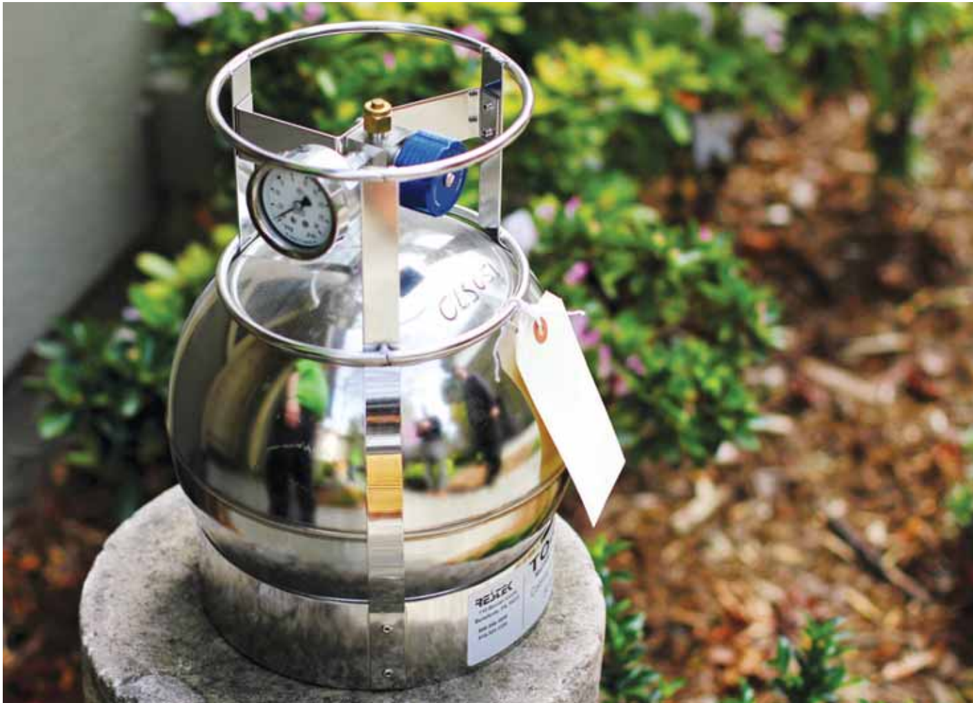
A summa canister holds an air sample.
