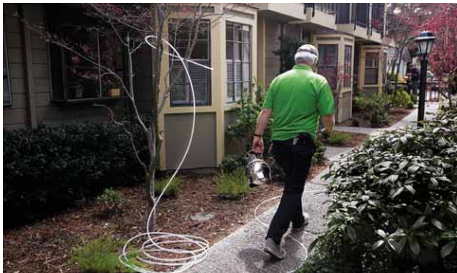
A Teflon tube collects a sample of outdoor air.
