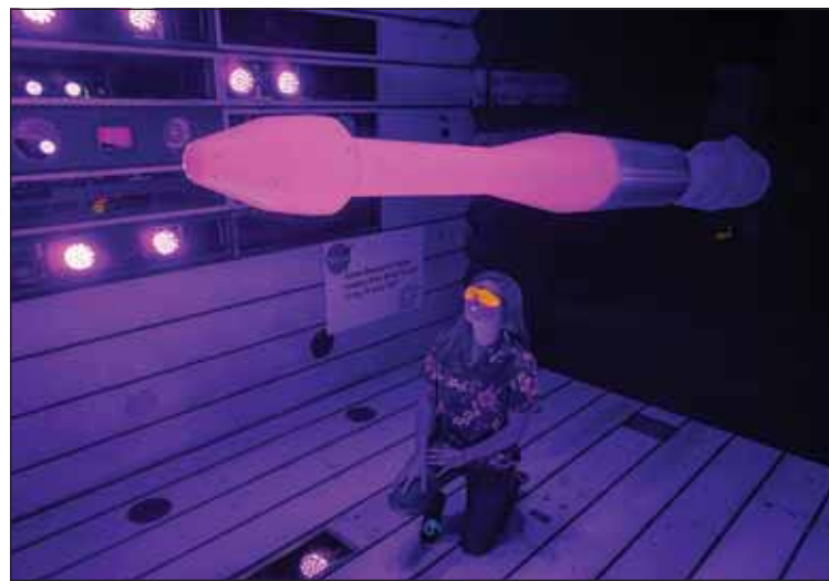
Nettie Roozeboom sits next to a model launch vehicle coated with pressure-sensitive paint, used to see how high-velocity pressure will affect aerospace vehicles.
